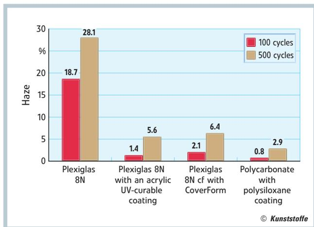
**Fig. 4. In the Taber abraser test, CoverForm parts yield values comparable to those for Plexiglas 8N parts coated with acrylic-based lacquers**
