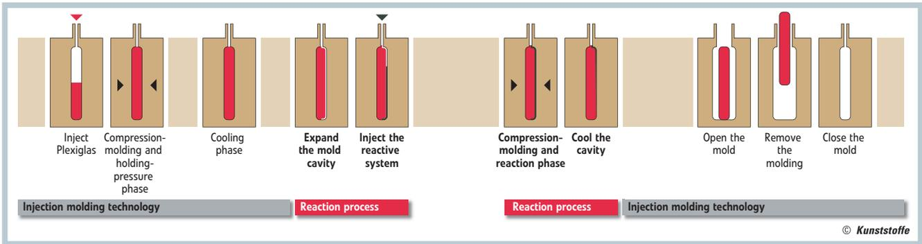
Fig. 1. Schematic representation of the CoverForm process
