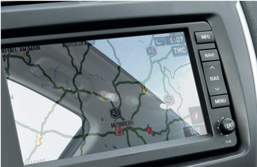
Fig. 1. Non-anti-glare surfaces on automotive dashboard instrument displays reflect the light and interfere with vision while driving
